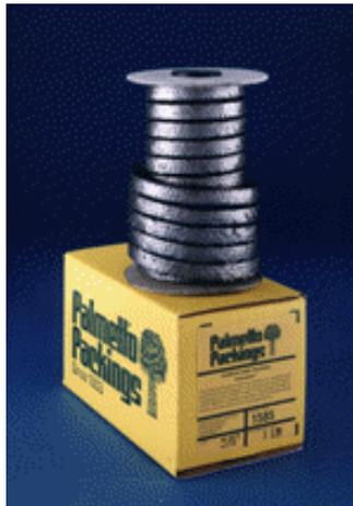
Interwoven™ braid of carbon fiber, Palcar™ is impregnated with graphite particles, which makes it ideal for boiler feed pumps, blowers, and driers. Temp. 1200°F (650°C) in steam, 650°F (345°C) in oxygen and 2400°F (1320°C) in reducing atmosphere. pH 1-14. Style 1585 exhibits extremely low coefficient of friction characteristics enabling dynamic equipment ease of operation and long trouble-free service life.
