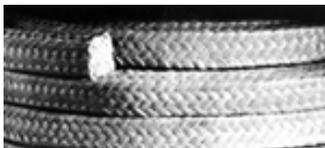
Interwoven™ braid of Aramid, the strongest synthetic fiber, and impregnated with TFE dispersion. Designed for abrasive applications where other packings don't measure up. Temp. 500°F (260°C) 3-11pH. Style 1350's inherent 'brute strength' characteristics enable it to withstand 'shearing and learing' action of abrasive applications.
