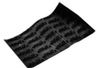
2970 is the direct replacement for asbestos sheet gasketing. Manufactured of predominantly Aramid Filament with premium NBR binders assures long shell life vs. asbestos sheet. Style 2970 is soft and compressible and is highly recommended for such applications as pipe flanges, mixers, ovens, kettle, manifolds, digesters, tanks, columns and pumps. Temp. 750°F (399°C). Leachable Chloride content is less than 100 ppm which helps prevent flange pilling.
