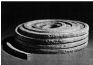
Palmetto 1392 is the direct replacement for TFE/Asbestos. Predominately Kynol\* composite (Quadrasyn) construction assures longer service life with reduced maintenance and subsequent downtime! Typical applications include stock pumps, beaters, Jordans, hydropulpers, hydroliners, blenders, dome lid gaskets (available in rectangular cross-sections). Temp. 500°F (260°C) 2-12 pH.
